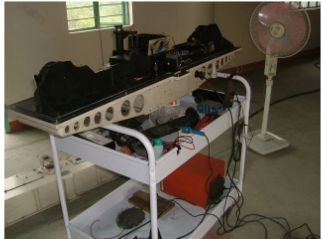
Photo. 3 Repair and checks of Dobson in penthouse.
