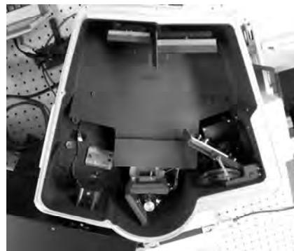
Photo. 1 Spectral sensitivity calibration system using iHR320 spectrometer.
