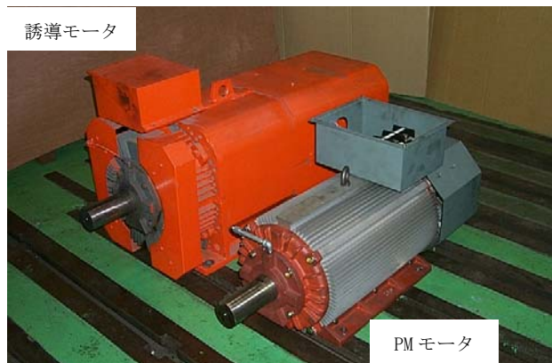
図1 110[kW], 1800[r/m]機の比較 Fig.1 Size comparison between IM and PMM
