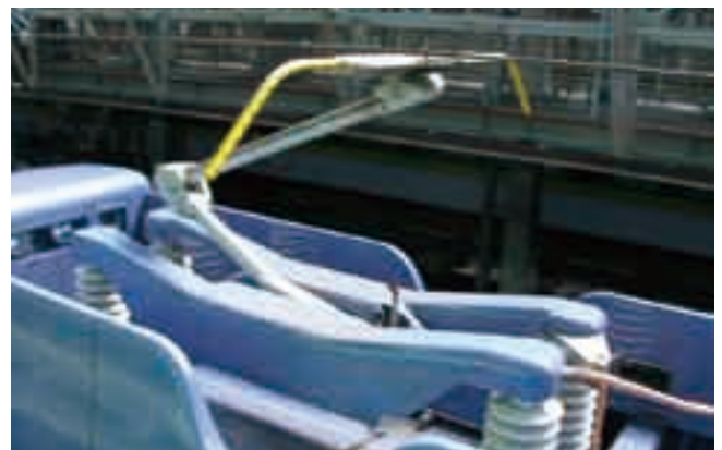
■ 図3 WPS208形パンタグラフ(反なびき方向) Fig.3 Appearance of pantograph WPS208 (Knuckle backward direction)
