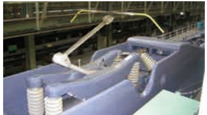
■ 図2 WPS208形パンタグラフ(なびき方向) Fig.2 Appearance of pantograph WPS208 (Knuckle forward direction)
