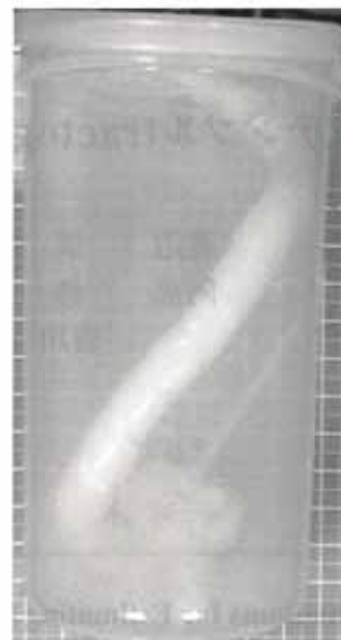
Fig. 2 Phantom of bundled polyester yarn (spirally twisted).
