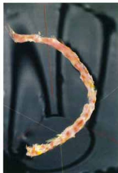
Fig. 4 Tractography of the polyester yarn phantom (spirally twisted).
