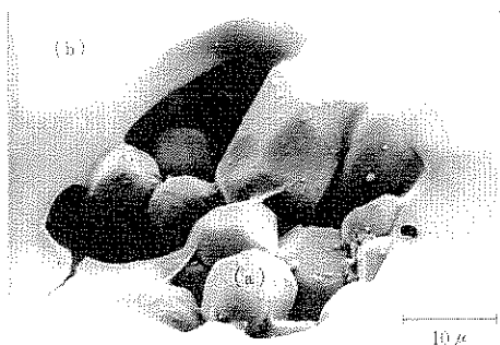
Fig. 12 Example of broken-film of acrylic resin on the phosphor particles. (a) acrylic resin film; (b) phosphor particle.
