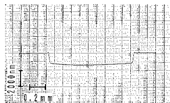
Fig. 8(b) Recording chart of surface profiler for spot-etching on synthetic diamond "Sumicrystal" surface.
