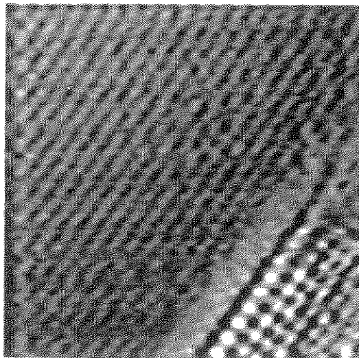
Fig. 9 STM image of Ni(111) after exposure to 100 L CO at 500 K. 56 \text{ \AA} \times 56 \text{ \AA} .
