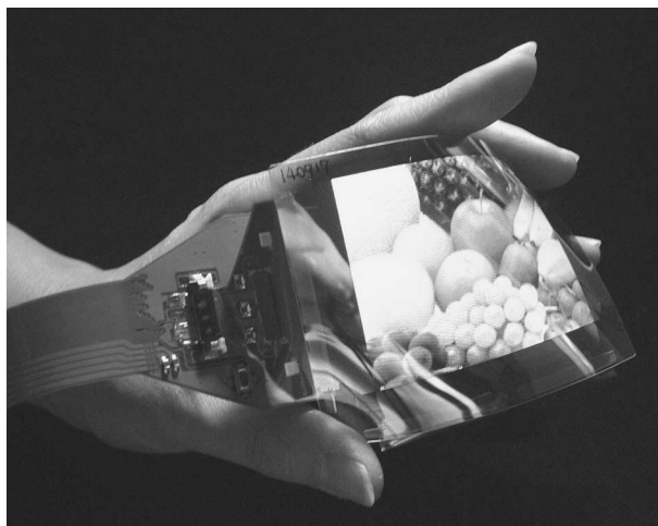
Fig. 1. Flexible OLED display 4) . This panel was demonstrated by Pioneer R&D group. Its active area is 62.4 × 46.8 mm, thickness is 0.2 mm and weights 3 gram with IC. Its resolution is 160 × RGB × 120 dots.
