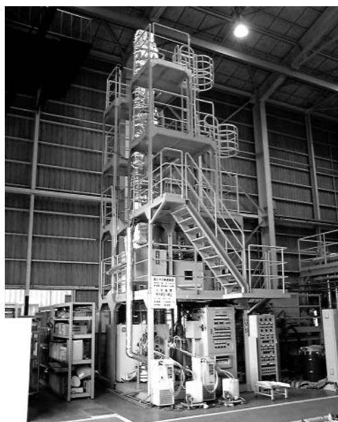
Fig. 4 Test apparatus of continuous PET depolymerization process The figure shows an external view of the laboratory apparatus for methanolysis with supercritical methanol process.
