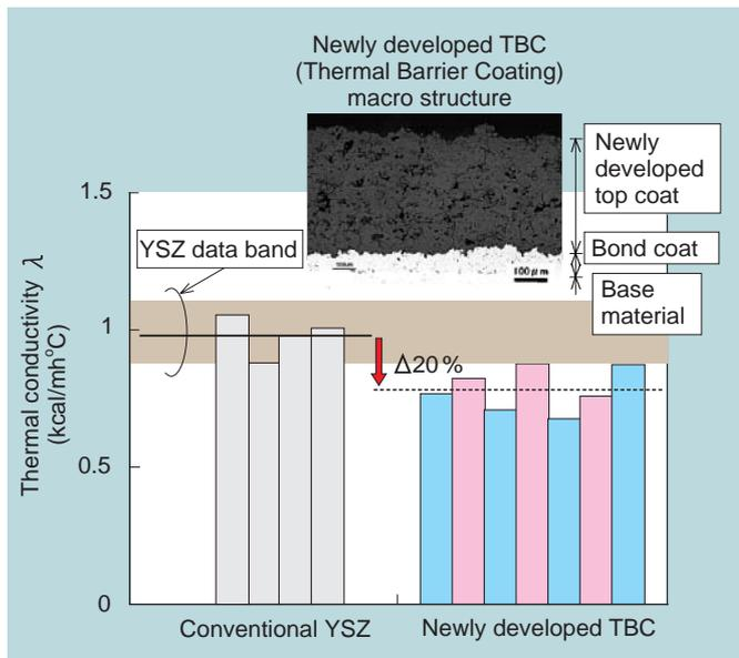
**Fig. 8 Results of measuring coefficient of thermal conductivity of newly developed thermal barrier coating**
