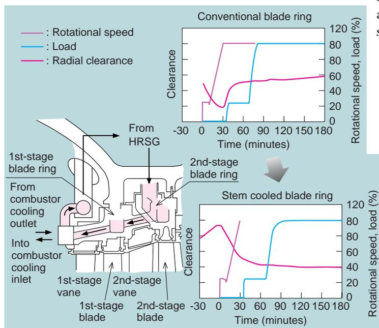
**Fig. 3 System and structure of the stem cooled blade ring**
