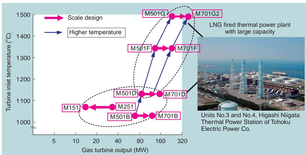
**Fig. 1 History of MHI's large frame commercial gas turbines**
