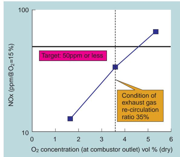
**Fig. 7 Results of atmospheric-pressure combustion test of new concept combustor**
