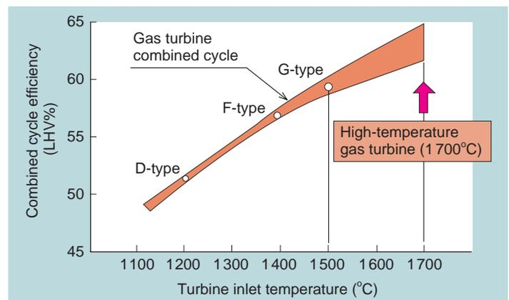
**Fig. 6 Combined cycle thermal efficiency VS. Turbine inlet temperature**
