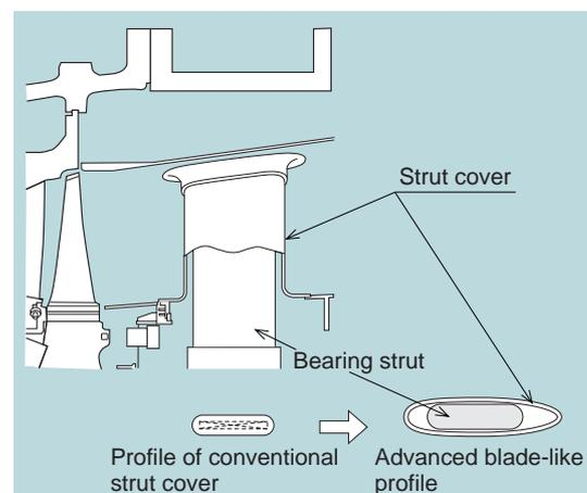
**Fig. 4 Profile of advanced exhaust strut cover**
