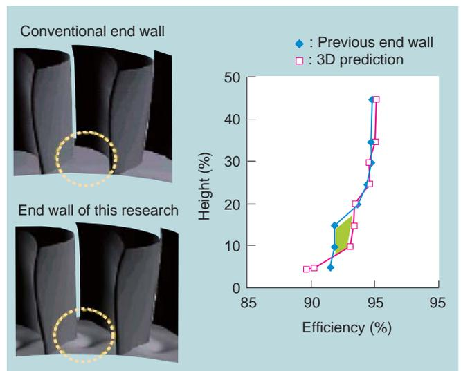
**Fig. 9 Profile and effect of three-dimensional end wall**
