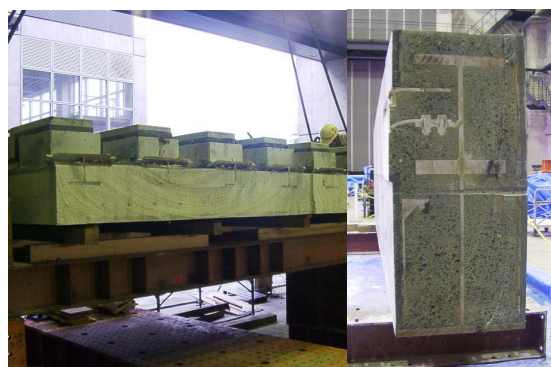
Photo 1 スラブ (左) と主桁 (右) の充てん状況 (Cutting Plane of Slab and Main Girder)
