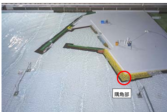
Photo 1 多方向不規則波実験状況 (Hydraulic model test using multi-directional random waves)
