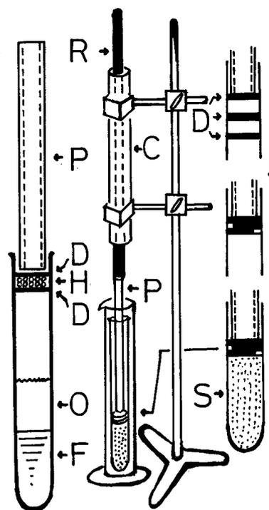
**Fig. 1.** Equipment for Plunger Top Filtration Method
