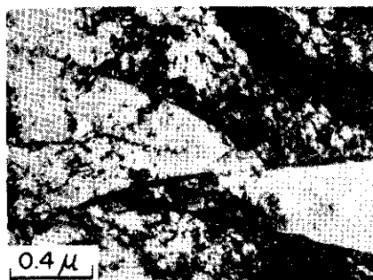
(a) Solution treated(820°C×1h A. C.)
