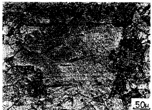
Photo. 4 A coarse grain produced by reheating to 1150°C and 6% rolling at 900°C in Nb-steel
