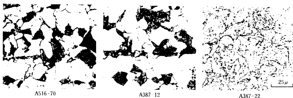
Photo. 1 Optical micrographs of base plates ( \frac{1}{2} t )
