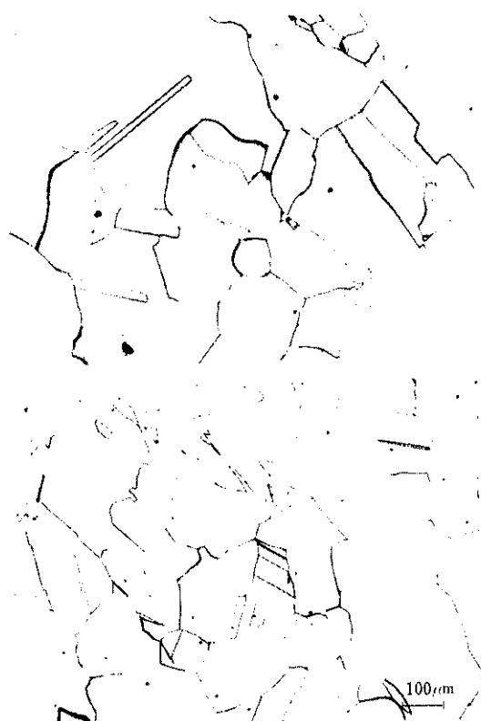
Photo. 6 An example of grain size for 265mm thickness forged shell
