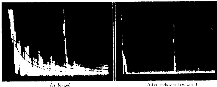
Photo. 5 An example of CRT figures of as forged and after solution treatment
