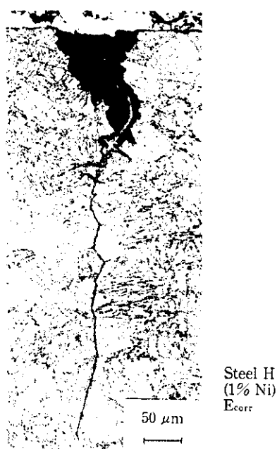
Photo 9 Typical crack observed on steel tested under E_{corr} in 3 000 ppm H_2S solution
