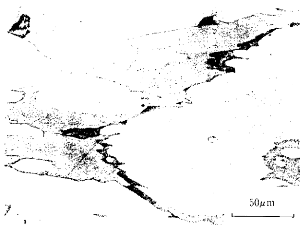
Photo 4 Crack initiation at austenite/delta-ferrite phase boundary
