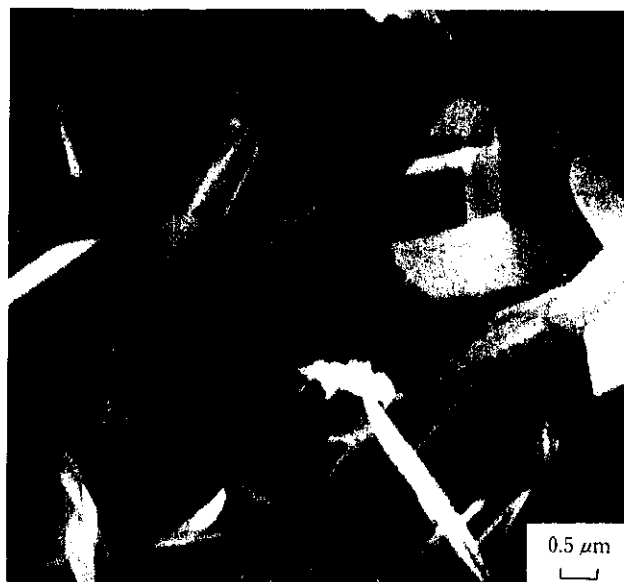
Photo 1 SEM photograph of tobermorite crystal
