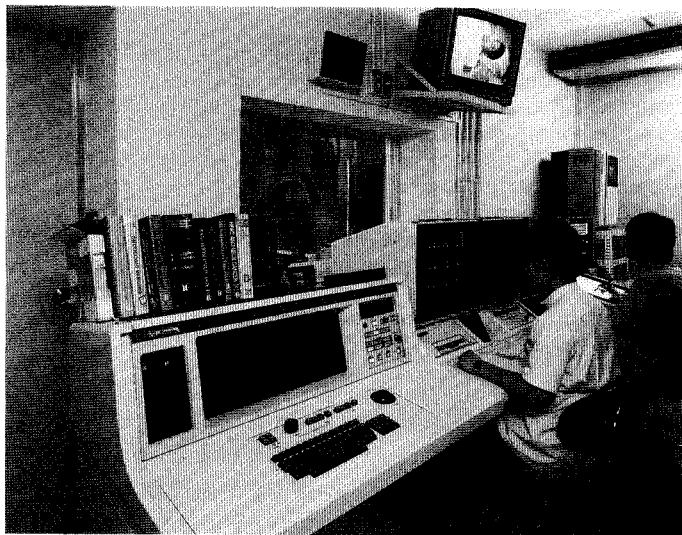
Fig. 2. CT Simulator (Operating room). CT operating console, multi-image monitors and treatment planning console.
