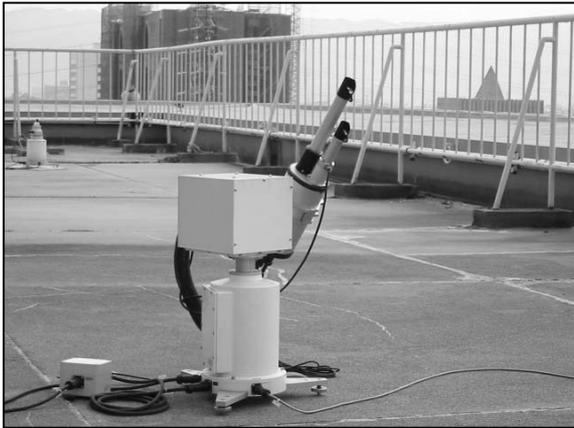
Figure 1: Sky-radiometer : POM-100P at Higashi-Osaka.
