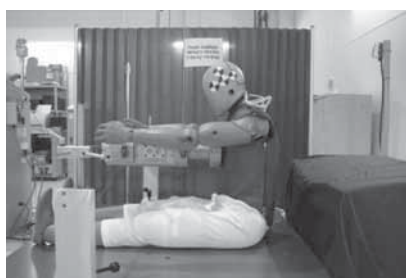
Fig. 2 Setup of thorax impact test
