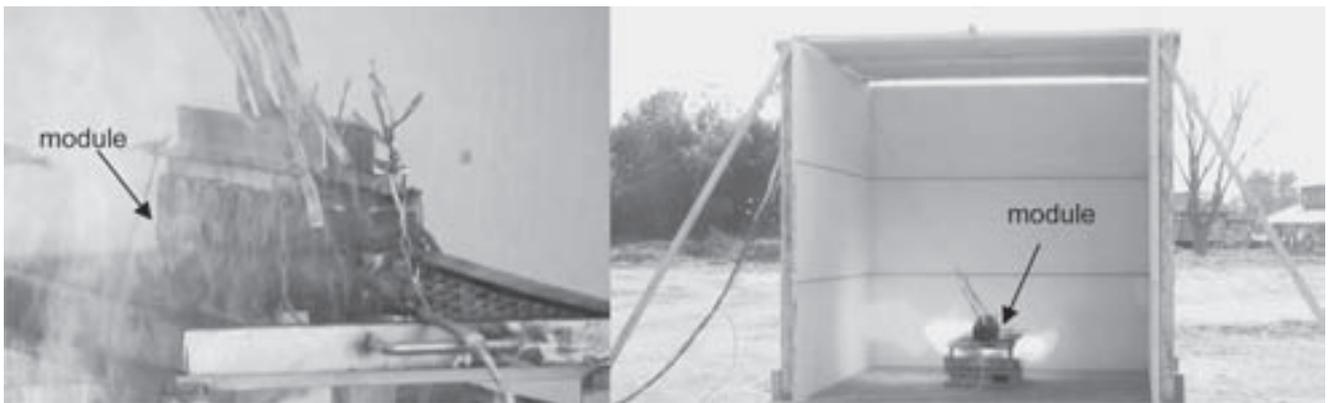
Fig. 4 Situation of bonfire test
