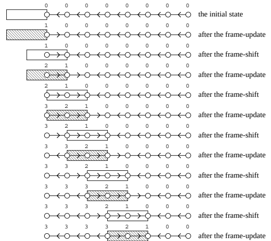
図 1 1次元の場合の枠の移動方法と更新状態を表すグラフ Fig. 1 Frame shifting method and updating state of unknowns in the one dimensional case.
