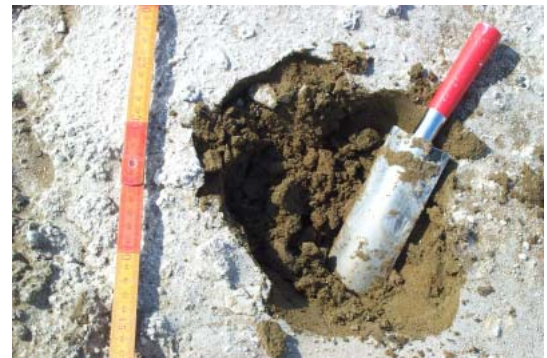
Photo 1 仮置き状態の発生土 The Soil of Reclaimed Land by Construction of Under-ground Tank
