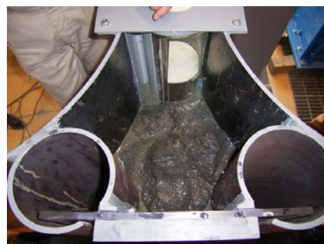
Photo 4 遮水材の充填状況 Barrier System Model filled with Barrier Materials
