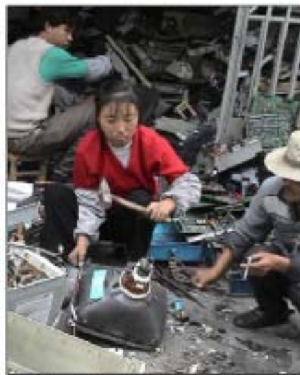
Dismantler cracking a monitor to remove the copper yoke. The rest of the CRT is dumped. © BAN
