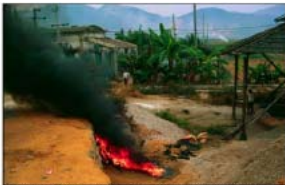
Open burning of wires and other parts are common to recover metals such as steel and copper. Dioxins and furans can be expected due to the use of PVC and brominated flame retardants. © BAN
