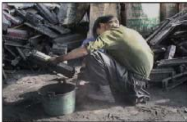
Worker without respiratory protection brushing carbon black toner from printer cartridge into bucket. © BAN
