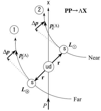
Fig. 5. The momentum transfer  $\Delta \mathbf{p}$  and the orbital angular momentum  $\mathbf{L}$  in the near-side and far-side collisions for the  $pp \rightarrow \Lambda X$  collisions.
