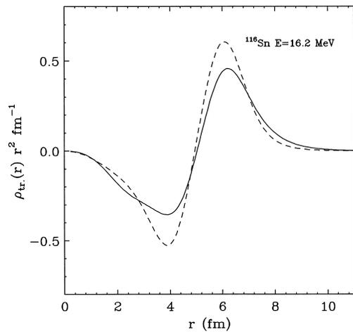
Fig. 2. Microscopic RPA (solid line) and collective model (dashed line) transition densities in  $^{116}\text{Sn}$  at the resonance energy  $E = 16.2$  MeV.
