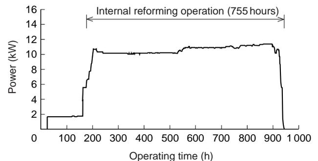
**Fig. 8 Result of Pressurized Internal Reforming 10 kW Module Operation: Continuous operation for 755 hours with methane reformation using internal heat generation**
