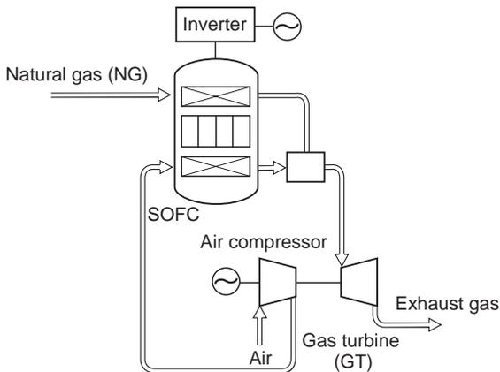
**Fig. 2 SOFC + Gas turbine System**
