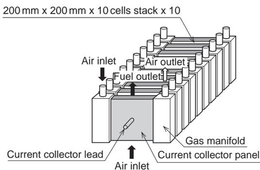
**Fig. 10 Structure of MOLB Type SOFC**
