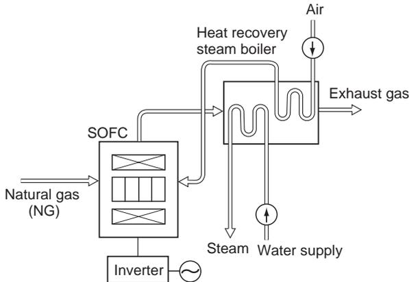
**Fig. 1 SOFC + Heat Recovery System**
