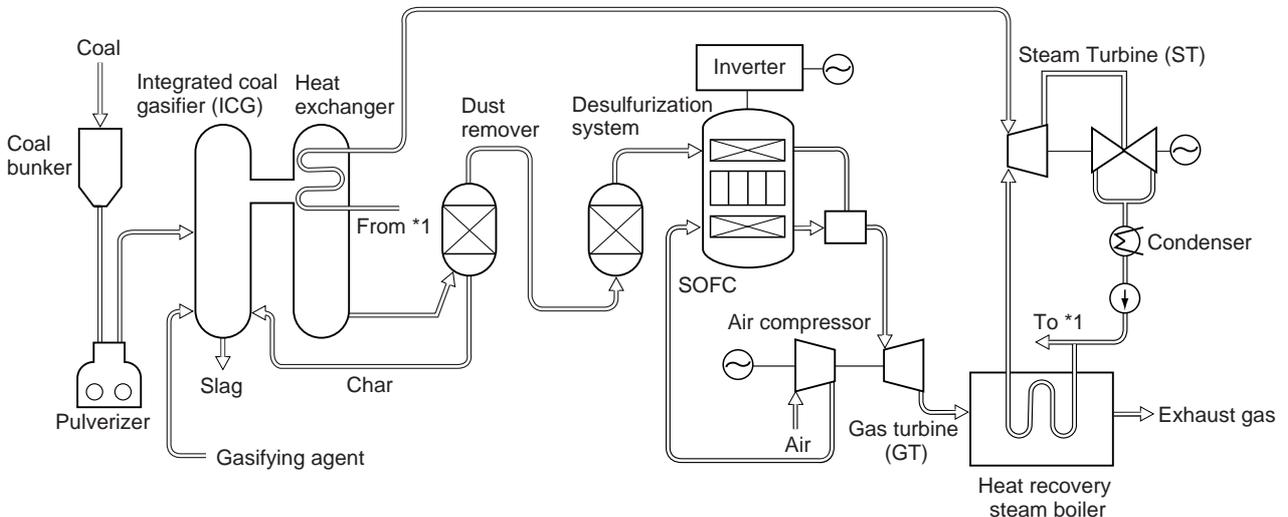
**Fig. 4 Combined Cycle Power System of Coal Gasifier + SOFC + Gas turbine + Steam Turbine**
