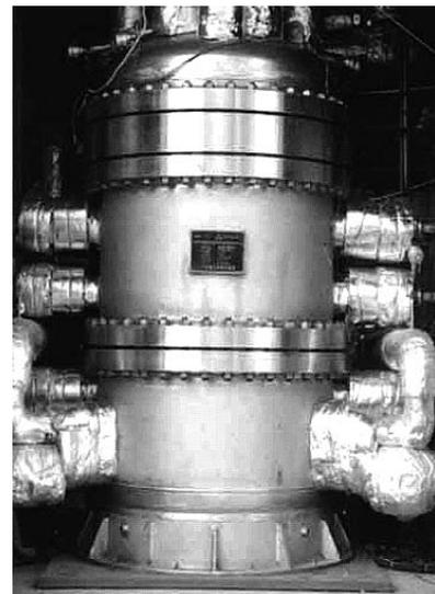
**Fig. 7 Appearance of Pressurized Internal Reforming 10 kW Module**
