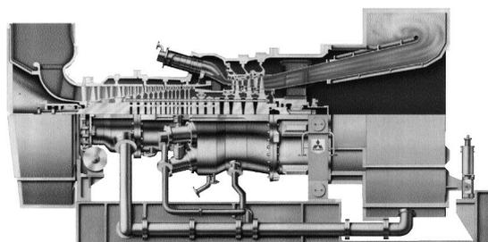
**Fig. 15 10 MW Class Gas Turbine (MF-111)**
