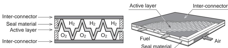
**Fig. 9 Structure of MOLB Type SOFC**
