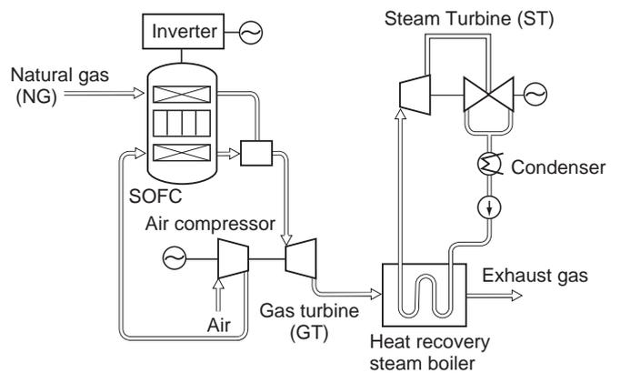
**Fig. 3 Combined Cycle Power System of SOFC + Gas turbine + Steam Turbine**
