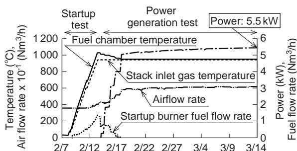
**Fig. 12 Test Results of "Thermally Self-supporting Module"**
