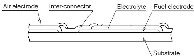
**Fig. 5 Tubular Sintering Type SOFC Cell Tube Structure**
