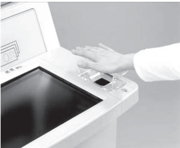
Figure 4 Contactless palm vein pattern authentication for ATMs.
