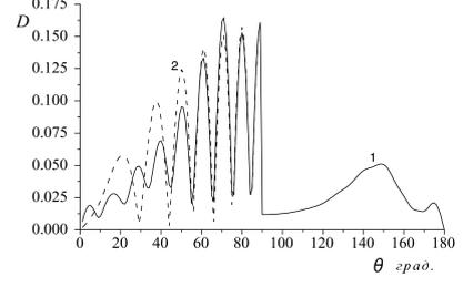
Fig.4 Far field pattern:  $kc = 24$ ,  $kl = 20$ ,  $\gamma = 89^\circ$ : 1 - semi-infinite truncated cone; 2 - semi-infinite cone.
