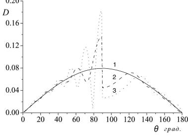
Fig.3 Far field pattern for semi-infinite truncated cone:  $kc = 24$ ,  $\gamma = 89^\circ$ : 1 -  $kl = 0.01$ ; 2 -  $kl = 5$ ; 3 -  $kl = 10$
