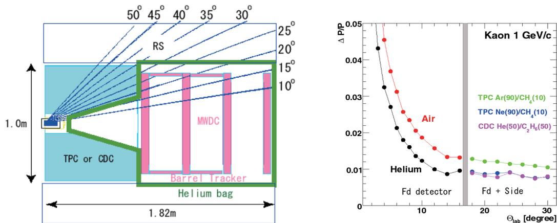
Figure 7: Schematic view of the tracking system (left) and the total momentum resolution  $\Delta P/P$  as a function of laboratory angle for a 1-GeV/c kaon (right).
