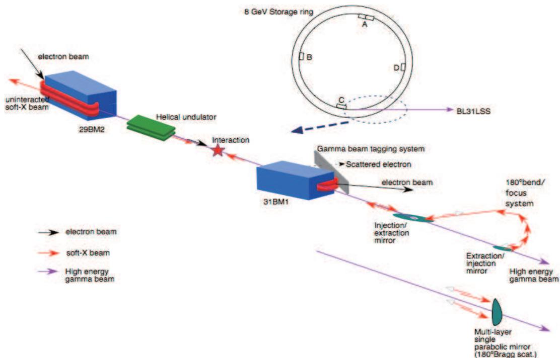
Figure 5: Schematic view of the X-ray re-injection.
