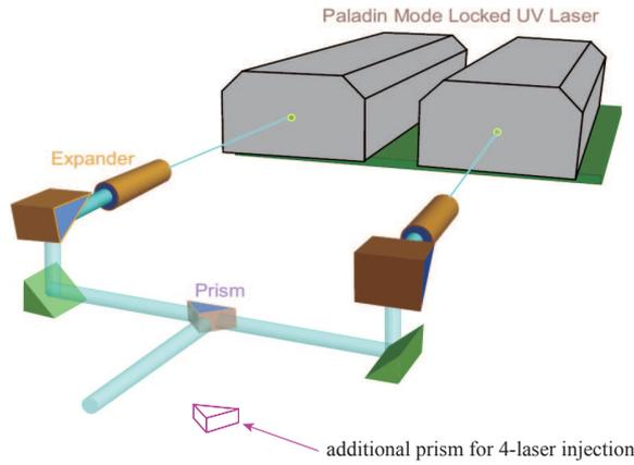
Figure 2: Two laser injection system tested at BL33LEP.
