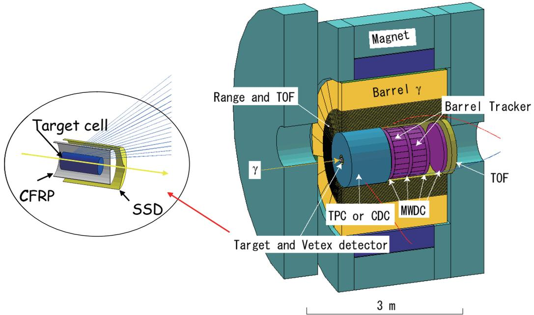
Figure 6: LEPS2 spectrometer with E949 solenoid magnet.
