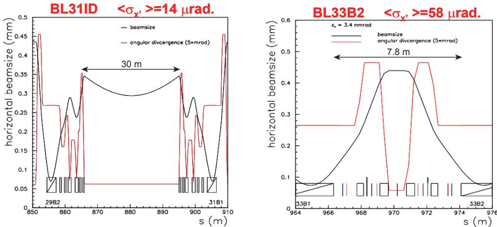
Figure 3: Comparison of the electron beam divergence for BL311D and BL33LEP.
