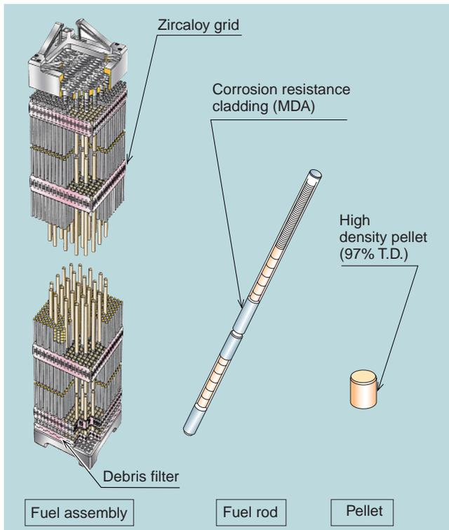
Fig. 6 Outline of structures of fuel assembly and fuel rod
