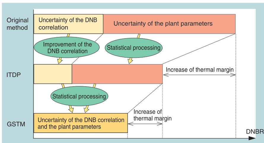
Fig. 5 Outline of expanded allowance due to improved thermal design
