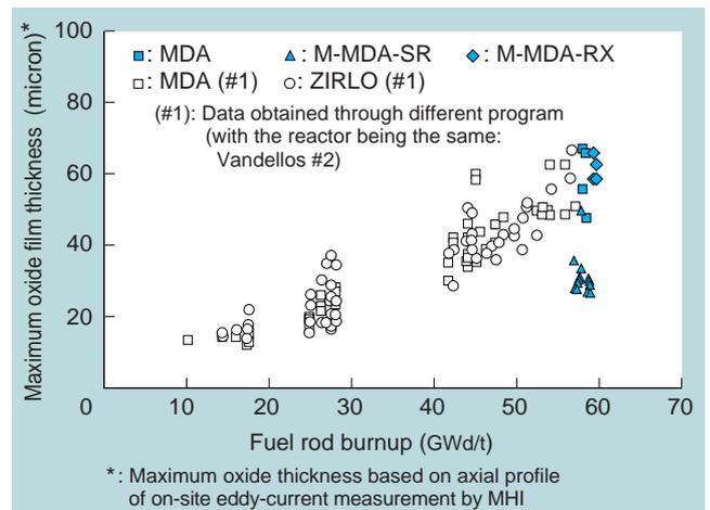
Fig. 7 M-MDA corrosion data in reactor
