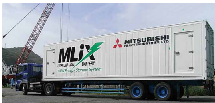
Figure 2 ESS during transport by trailer
