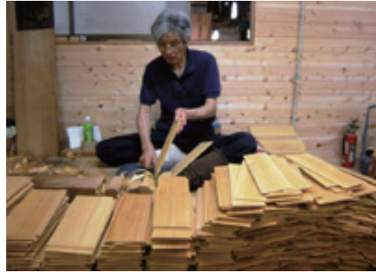
Selected Conservation Techniques: Production of roof shingle Holder: KURIYAMA Mitsuhiro
