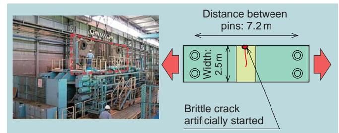
**Fig. 7** Tester and test hull to measure resistance to large scale brittle crack propagation
