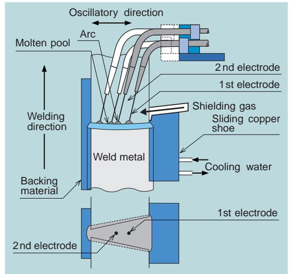
Fig. 10 Schematic drawing of tandem-electrode VEGA welding method
