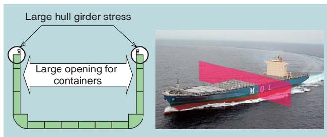
**Fig. 5** Structural characteristics of container ship (midship section)
