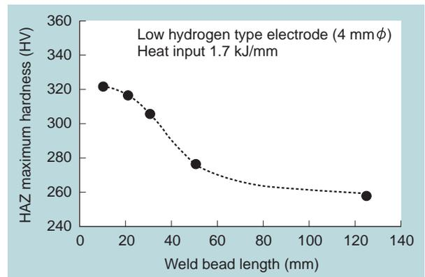
Fig. 14 Results of HAZ maximum hardness test
