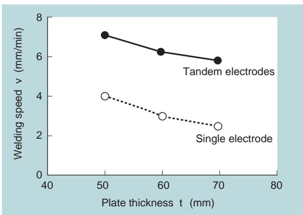
Fig. 11 Relation between welding speed and plate thickness
