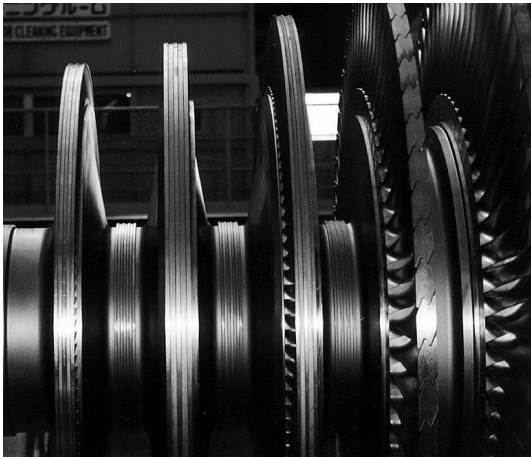
Fig. 5 Appearance of application of integral shroud blades (ISB)
