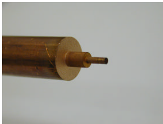
Fig. 4 Sample of shaft machining by WEDM
