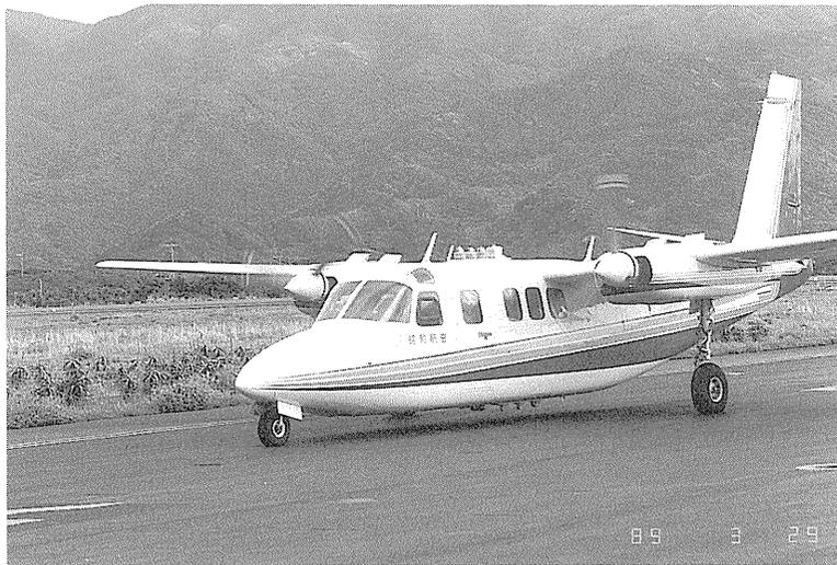
Photo 2.1.2 Aerocommander-685 equipped with various radiometers.
