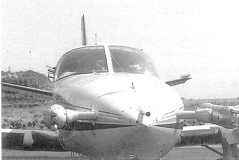
Photo 2.1.1 Cessna-404 equipped with various cloud-physics probes.
