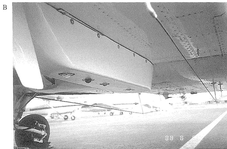
Photo 2.2.1 A pair of radiometers installed on the top (Panel A) and bottom (Panel B) of an aircraft fuselage, to measure the downward and upward radiative fluxes, respectively.
