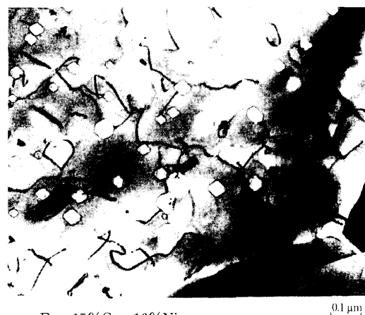
Fe-15%Cr-16%Ni neutron irradiated (JMTR) ( 8 \times 10^{21} n/cm 2 , 480°C)
