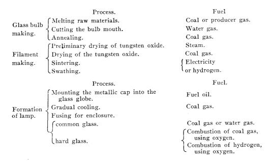
In the process of fusing the glass for closing the lamp mouth, the author found that the operation velocity was higher by about 15–20% when employing water gas only than when mixed with coal gas.
