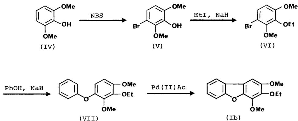
Scheme 1 Synthesis of eriobofuran ethylether (**Ib**).
