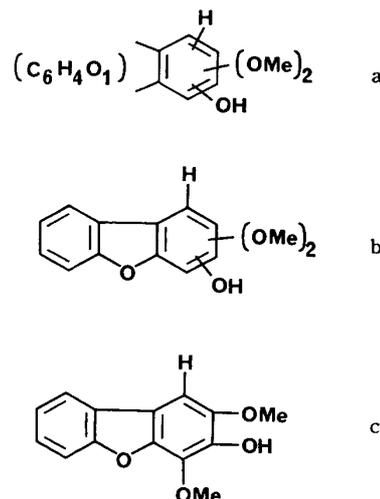
Fig. 2 Partial and total structure of eriobofuran.
