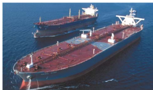
Figure 1: The approach phase of a lightering operation.
