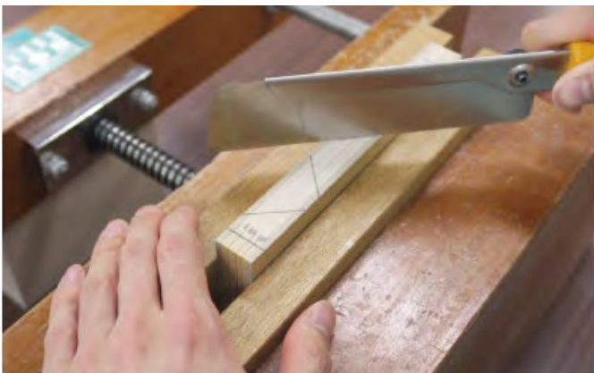
Remove the cover and make saw cuts in the spine.
