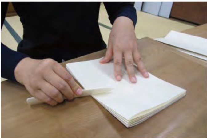
Folders can also be used to fold a large number of sheets of paper or thick paper.
