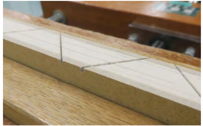
To prevent the linen cord from falling out, alternate the direction of each cut.
