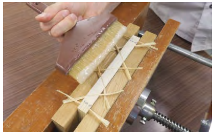
After applying adhesive, the linen cord is embedded in the groove, and then additional adhesive is applied to the spine to harden it.
