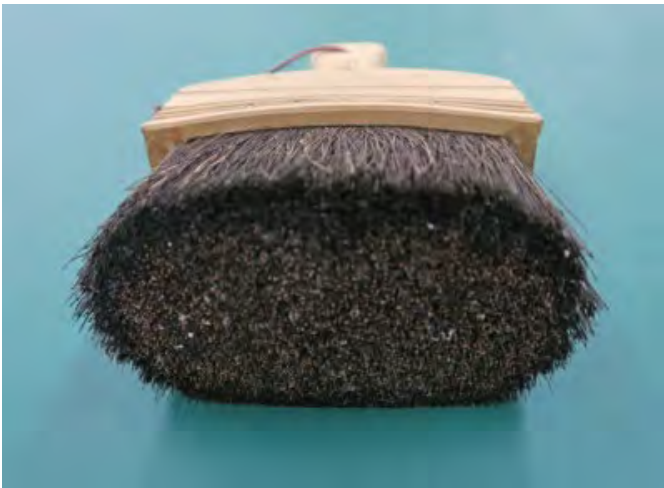
The bottom of a pounding brush is flat. Pounding is performed by using the flat side of this brush, shifting the location little by little to pound the entire lining evenly.
