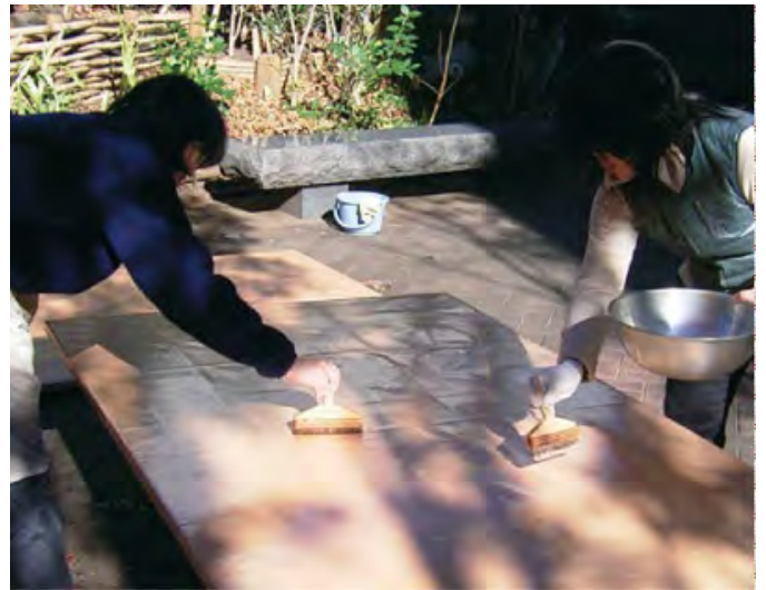
Coating the karibari board with persimmon juice is done outdoors.
