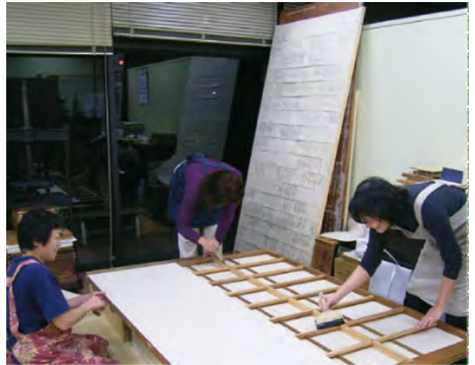
Attaching the first layer of paper to the frame. Several more layers will be added.
