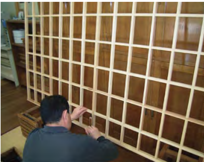
Making a frame for a karibari board.
