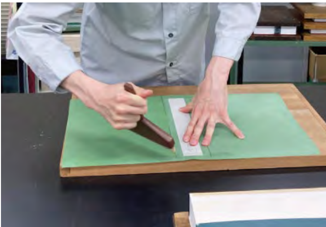
Applying paste on the bookbinding cloth with a brush.
