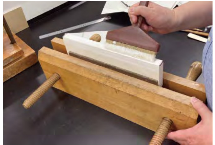
Fixing the spine of a book by applying adhesive with a brush.
