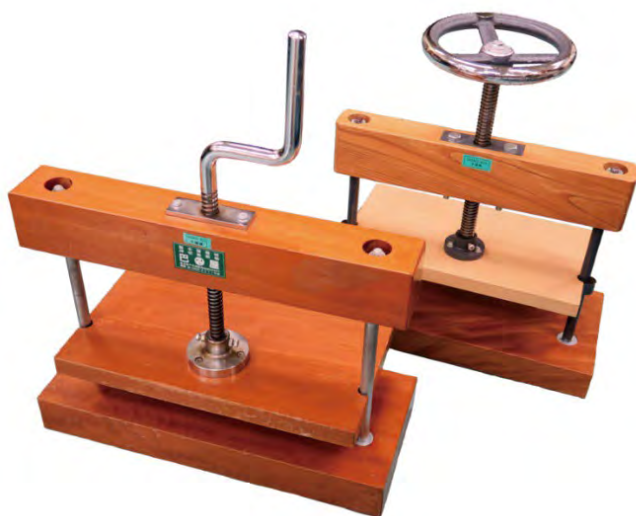
Turning the handle raises or lowers the top board.
