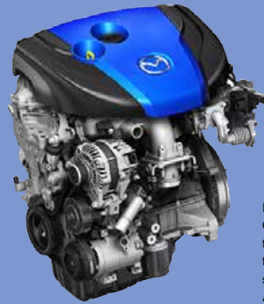
The SKYACTIV-D is a clean diesel engine commercialized by Mazda Motor Corporation. Utilized clean combustion technology results from a NEDO project with industry-university cooperation between Hiroshima University and others.
