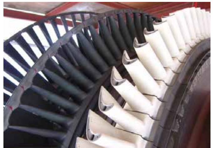
Hitachi, Ltd. developed gas turbine blades with high-durability heat-resistant coating.
