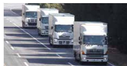
Image of four large-sized trucks in a test of automatic speed and vehicle distance control.
