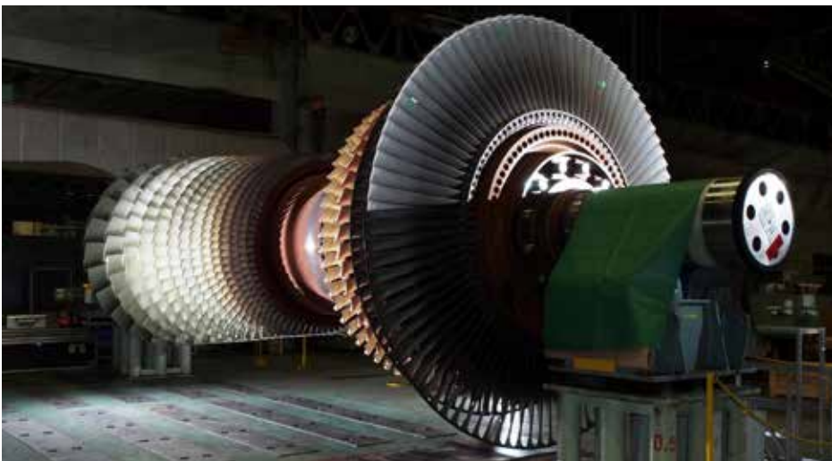
1500°C-class gas turbine rotor developed by Mitsubishi Heavy Industries, Ltd..
